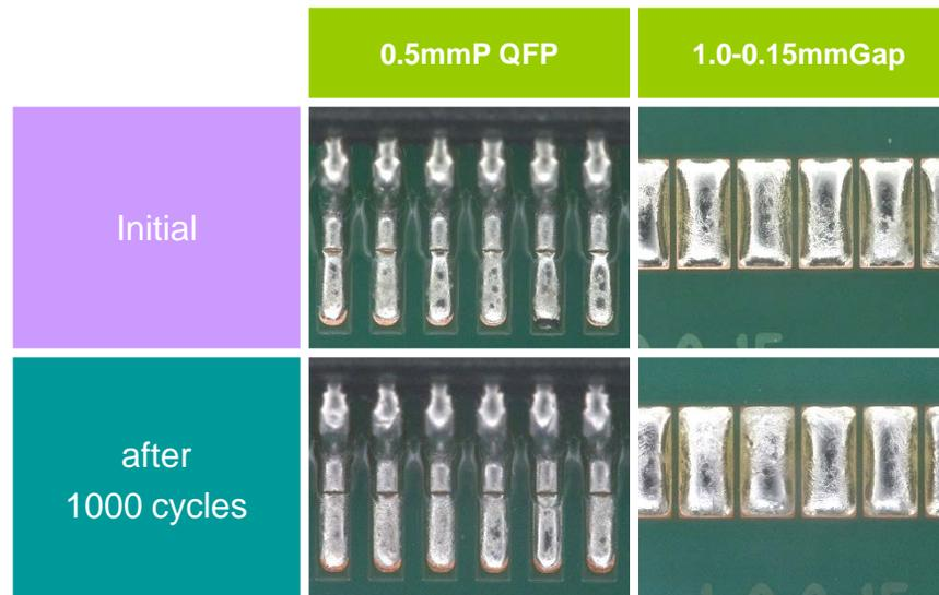
No cracking has occurred in the flux residue between the leads or electrodes, even after thermal cycling of -30/+80 °C x 1000 cycles.
