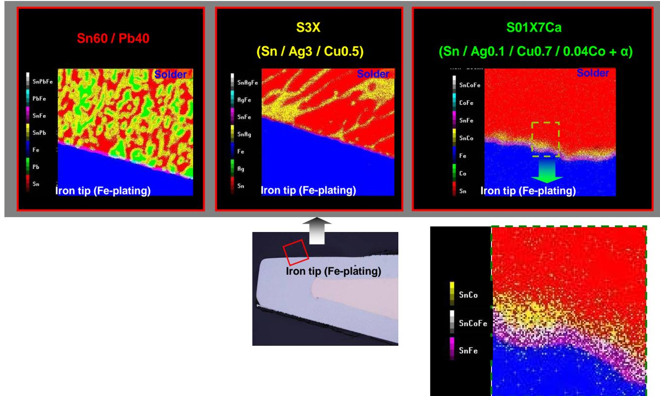
When using Sn60/Pb40 solder, tip erosion is minor, as Pb in the interface forms Pb-Fe compound, preventing Sn-Fe from dispersing Fe into the solder. Whereas in lead free solders such as S3X (SAC305), tip erosion is noticeable because Fe gets dispersed constantly into the solder. Having Co as its constituent, S01X7Ca and S03X7Ca alleviate tip erosion, with Co replacing Fe in Sn-Fe, and forming barrier layers of Sn-Fe, Sn-Co-Fe, and Sn-Co between Fe plating and the solder.
